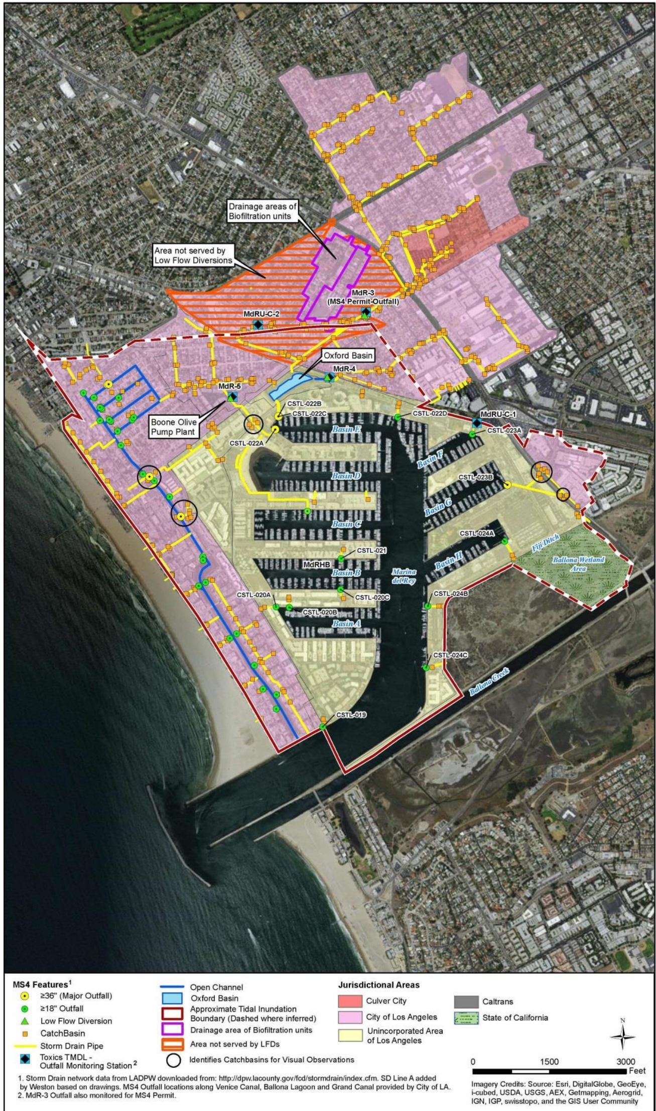
Figure 5-1. Extent of Tidal Influence, Major Outfalls and Catchbasins for Visual Inspection in the Mdr Watershed
