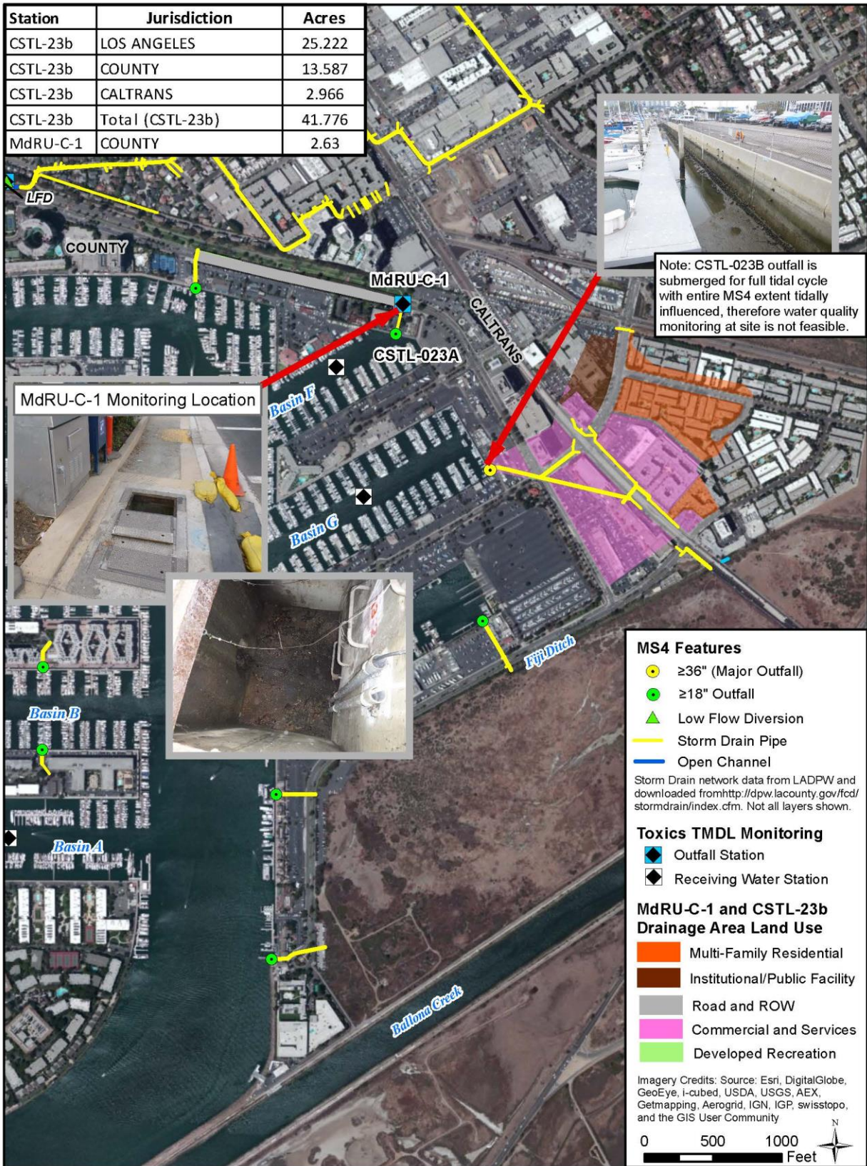
Figure 4-3. Outfall Station MdRU-C-1 (Toxics TMDL Monitoring) and Tidally Submerged MS4 Tributary to Major Outfall CSTL-023B
